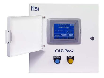
Cat-Pack provides remote monitoring of the compressor catalyst system, monitoring pre and post catalyst temperatures and differential pressure across the catalyst, O2 voltage and runtime. This data is then logged locally and provided as a local download, or can be transmitted as Modbus data to a central SCADA system.
